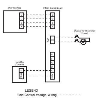
Fig. 14 - Control Voltage Wiring Connections
